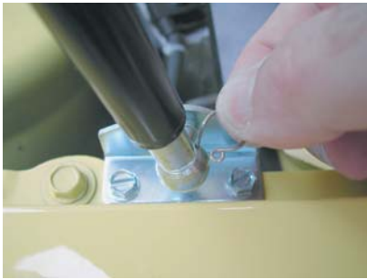
Insert clip into hole.
