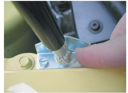
Rotate clip until it snaps onto shaft.
