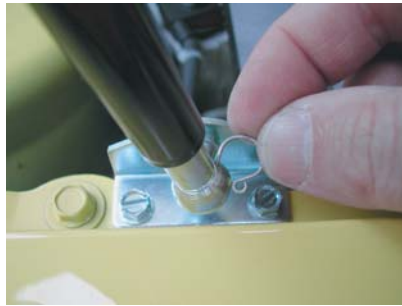
Slide clip down till it stops.
