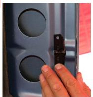
B. Using a center punch and a hammer, tap the center of the dot you just made (the indention will help guide the drill bit and keep it from wandering). Place bracket back in place to be sure it is still centered where it should be before moving to Step 6. Set bracket aside.
