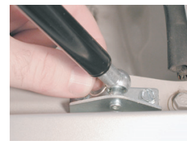
Slide clip down till it stops.
