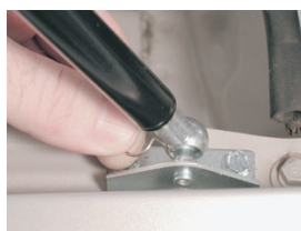
Insert clip into hole.
