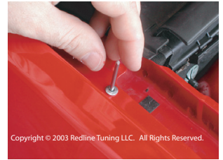
Test fit rivet in hole.
