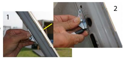
C. Using a center punch and a hammer, tap the center of the dot you just made (the indention will help guide the drill bit and keep it from wandering). Place bracket back in place to be sure it is still centered where it should be before moving to Step 5. Set bracket aside.
