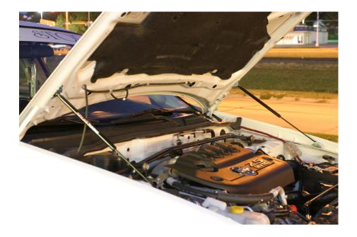
Check over the installation carefully to be sure each step was properly completed. Next check that each ball-stud socket is snapped securely onto the ball-studs.
