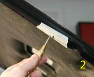
B. Using a center punch and a hammer, tap the center of the dot you just made (the indention will help guide the drill bit and keep it from wandering). Place bracket back in place to be sure it is still centered where it should be before moving to Step 5. Set bracket aside.
